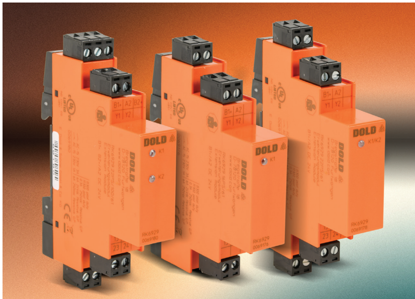
Figure 8: These Safety Extension Relays are rated for Category 3, PLe, SIL 3, but if they are used by themselves alone as a safety relay, it will be impossible to reach the required PL ratings.
