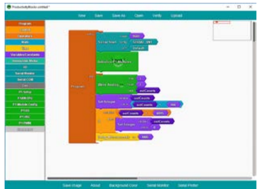
Figure 3: The addition of AutomationDirect ProductivityBlocks graphical programming software gives end users another accessible way to incorporate open source Arduino microcontroller functionality into their industrial projects.
