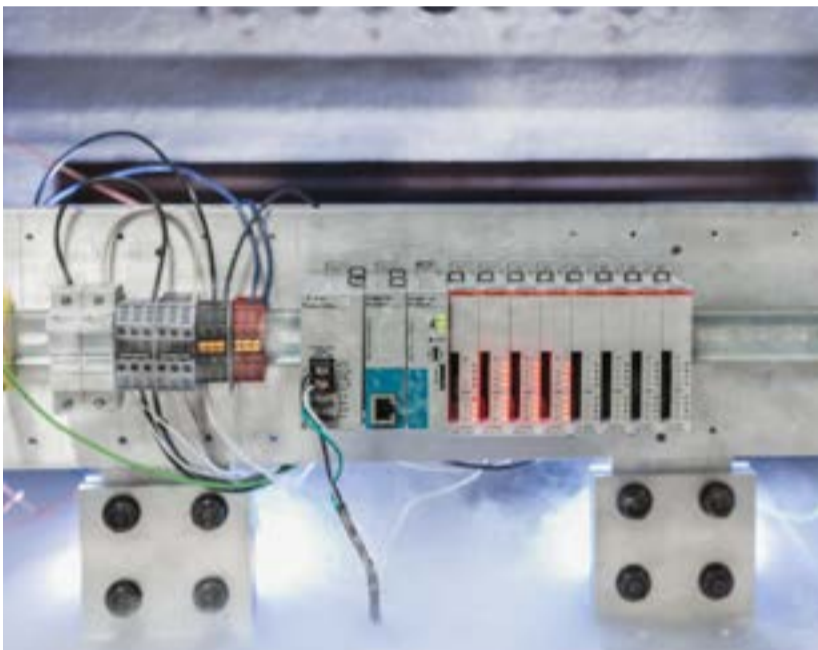
Figure 3: Unlike consumer-grade controllers, industrialized controllers like the AutomationDirect ProductivityOpen shown here, are tested in extreme conditions to ensure reliability in the field.
