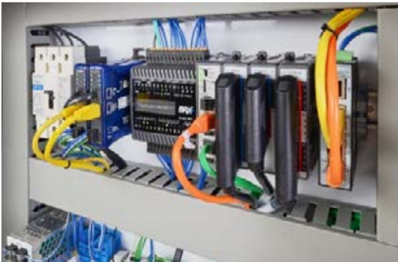
Figure 2: Next-generation PLCs, like the AutomationDirect BRX Series, are built from the ground up with OT and IT communication protocols, and the necessary security features, for enabling seamless data integration. With the free programming software, users can configure the BRX (with or without classic I/O) to also act as a data gateway
