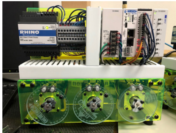
Figure 1: The AutomationDirect CLICK PLUS, shown here, is a modern micro-PLC enhanced with high-speed pulse train outputs and a straight-forward instruction set, making it practical, economical, and easy for users to implement motion control with open-loop stepper motors for applications of three axes or less.
