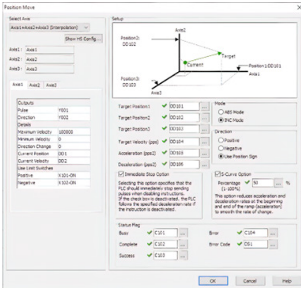
Figure 6: The “Position Move” instruction depicted here makes it straightforward for users to implement synchronized two-axis or three-axis combined movements, which are needed for many common machine automation applications.
