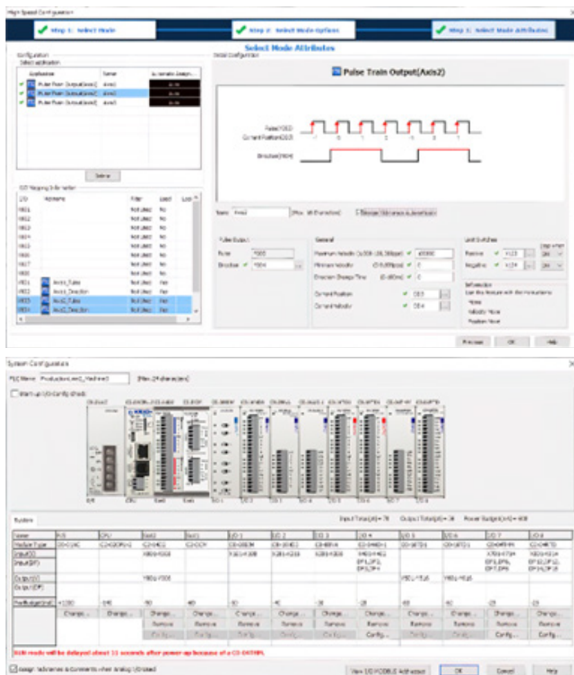
Figures 2 and 3: The AutomationDirect CLICK PLUS PLC development environment is intuitive and graphical, empowering users to rapidly define the hardware and high-speed discrete output configurations, and to coordinate them with stepper systems.
