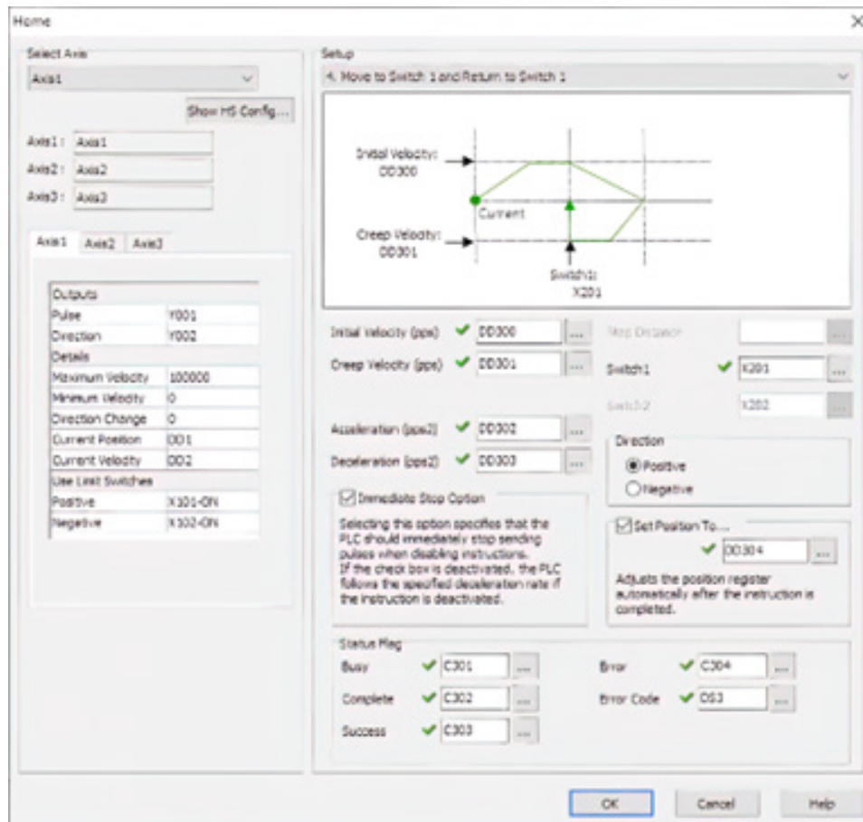
Figure 4: The “Home” instruction in the simplified instruction set includes the six most common standard homing methods, prompting users to select the necessary information.
