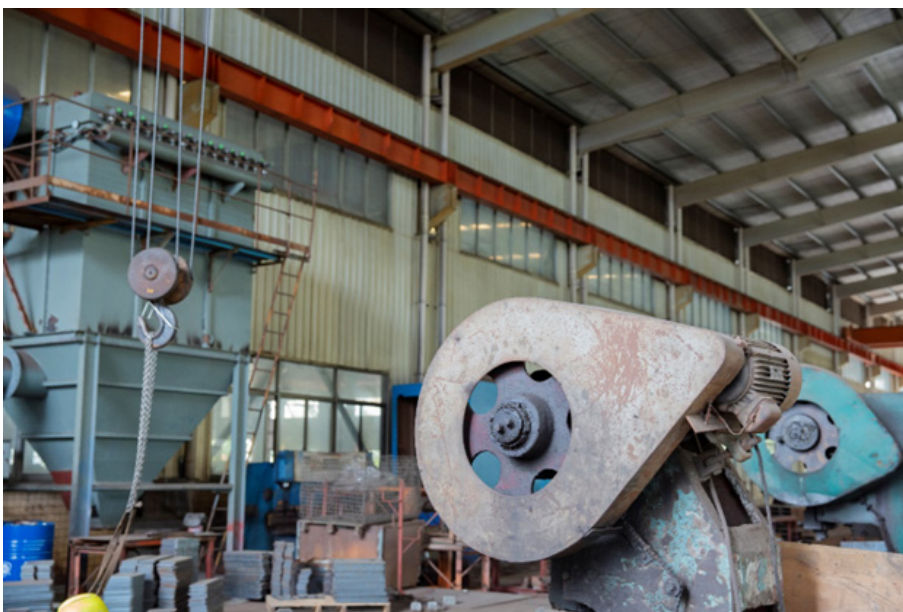
Figure 2: A high inertia load can cause regeneration even at a steady speed.
